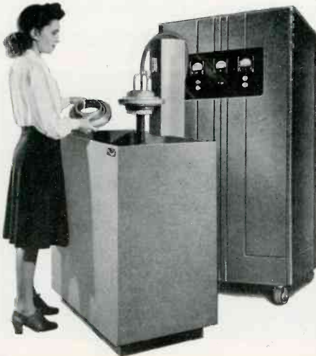
Inside hardening of aircraft engine raceway by induction heating
