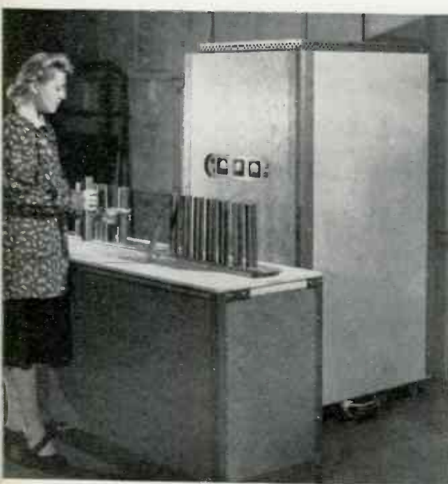
Above the incendiary bombs in this photograph were among those Doolittle dropped on Tokio. The girl is inserting bombs in a special heating coil for quick, multiple brazing operation, with induction heating.
