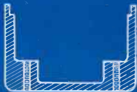
MACHINED ROD TO SPUN TUBING SAVING 50% BRASS
