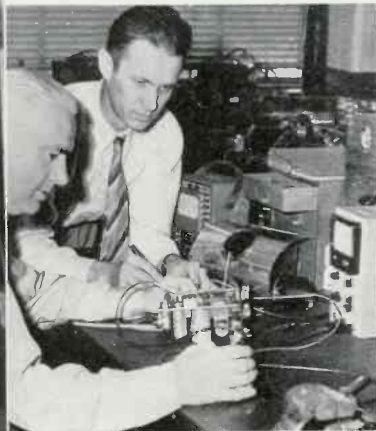
Electronic device for aircraft, developed by Minneapolis-Honeywell Regulator Co., measures ice forming on wings and operates de-icers at critical moment. Minneapolis-Honeywell is engaged in mass production of various electronic devices for war effort.
