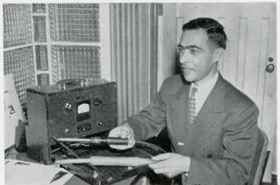
Latest improved form of the Moorhead-Berman electronic device which located shrapnel in victims of Pearl Harbor. Engineer Samuel Berman offered instrument in recent case of needle in child's heart
